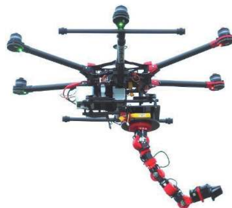
Fig. 14 Aerial manipulators with multi-DOFs [116]
