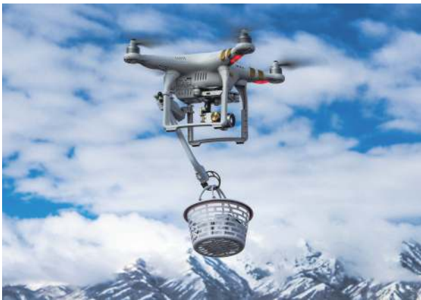
Fig. 9 Side robotic arm-kit compatible with DJI drones, registered trademark of GearWurx, re-printed with permission from GearWurx [105]
